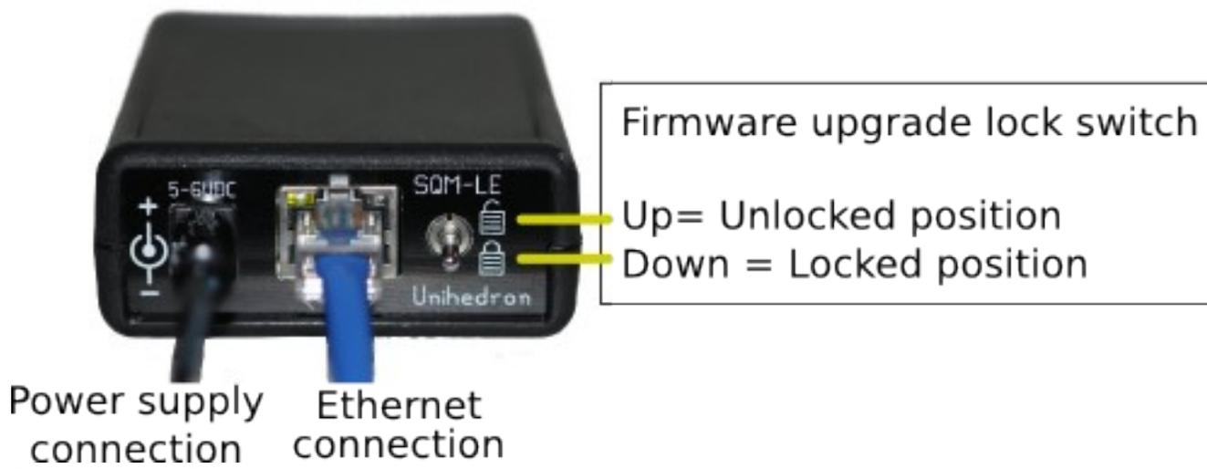
Power supply connection    Ethernet connection
